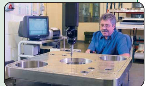
Inspection of a base plate.
