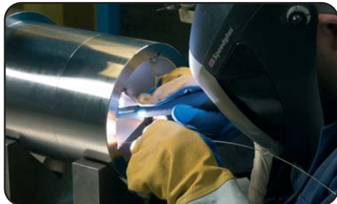
Welding a fuel stringer component.
